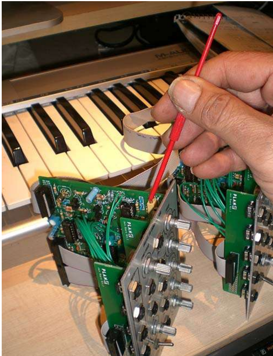
Figure 3 - Using a plastic pot tweaker to adjust the 1 volt/octave trim pot of a Rev 1.xx Model 15
